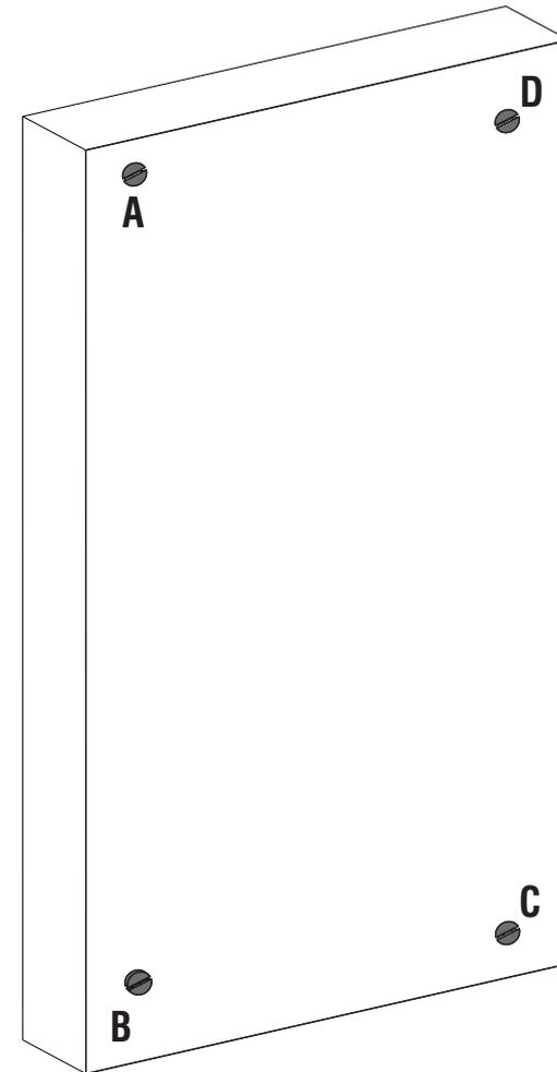
5. Align Key hole slots of COSEC COGNIFACE INTEGRA with the screws **A**, **B**, **C** and **D** on the wall and slightly slide it downwards as shown in **Figure 15** and **Figure 16**.
